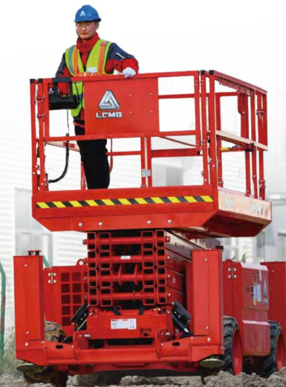
LGMG's micro scissors are ideal solutions for the low-level access and space restricted application job sites. Shorten overall machine length, lighter weight and compact design make the machine suitable for most elevators.
